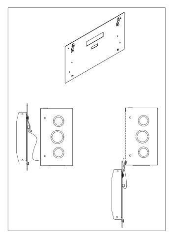
Figure 1-2 Hook Mounting the Display Unit
